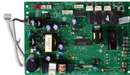
Main circuit board
